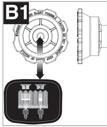
**Cone nozzle (blue - figure B1)** - The cone nozzle spray pattern is more concentrated. Use this nozzle for items that are too small for the fan nozzle. This is the spray nozzle that is identified as number 2 in the diagram on top of the sprayer.
